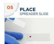
Place the spreader slide on top of the labeled slide in front of the blood droplet and hold at a 30° to 45° angle
